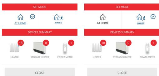
When the status is “absent” the “Away” mode is activated on the radiator screen.
