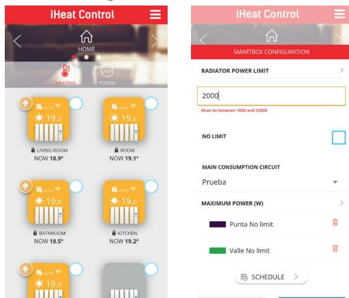
If you want to establish a priority for the emitters (Low, Medium or High), it can be configured within the options of each radiator, to do so click on the device icon, then on “more” and “configure”.
