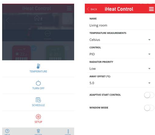
The control unit will first turn off the lower priority radiators, unless the difference between the set temperature and the measurement temperature is considerable, in order to guarantee an adequate temperature in all instances of the home.
