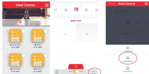
We will have a screen like the one shown below, in which we can program by day and by hour with the different modes (Comfort, Eco or Antifreeze). To do this, press on the day that we want to program and in “DEF TEMP” set the temperature that we want for each mode.
